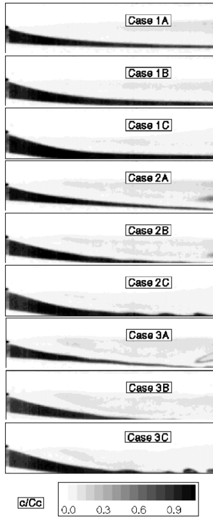
Fig. 3. Instantaneous mixing patterns in Plane 1 for Position O2 of the rotated (90°) cannula.
